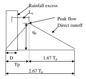
Figure 8.2: SCS triangular hydrograph
